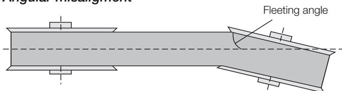
To check alignment, you will need a straight edge or, for long centre distance drives, heavy string. Line the straight edge or string along a machined face of both pulleys as shown on the picture below. Misalignment will show up as a gap between the face of the pulley and the straight edge or string. When using this method, make sure the distance between the groove edge and the outer rim of both pulleys is identical. Pulleys can also be checked for tilting with a spirit level.
