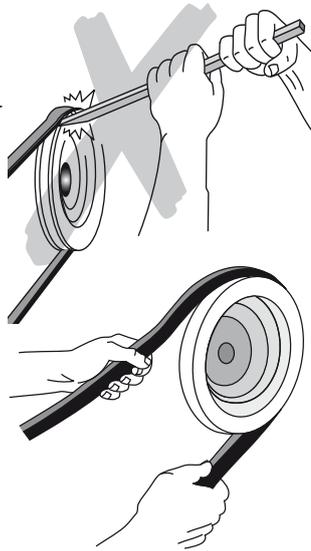
2. Remove old belts. Check them for unusual wear. Excessive wear may indicate problems with drive design or maintenance procedures.
