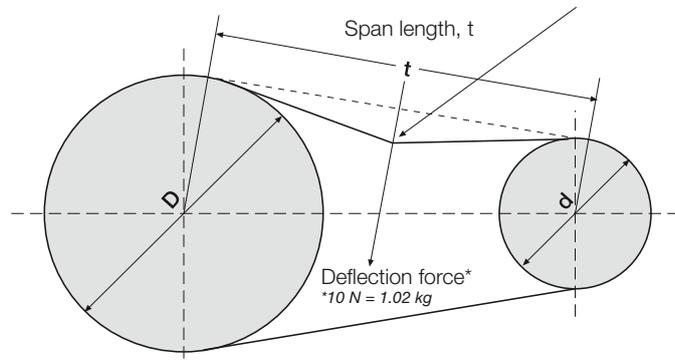
The final step is to check belt tension, and, if necessary, retension the belt. Note that retensioning is not recommended for synchronous belts. If too little tension is applied, V-belts may slip. The correct tension is the lowest tension at which the belts will transmit power when the drive is at full load.
